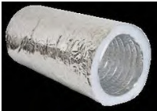
IFD-PD Polyester insulated flexible duct double layer alu foil duct + polyester +alu foil jacket temperature rating -30 to 150°C fire resistant standard length: 10m
