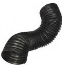
FC-CFD Material : PVC Constructure: double layers PVC + metal wire Temperature rating:-30 to 150°C Standard length: 10meters
