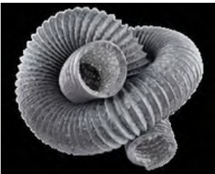
CFD PVC combine flexible duct constructure: PVC+PET +alu foil temperature rating -30 to 150°C fire resistant standard length: 10m
